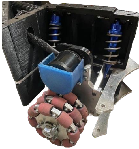
Fig. 3 . Suspended gearbox with omni-wheel
