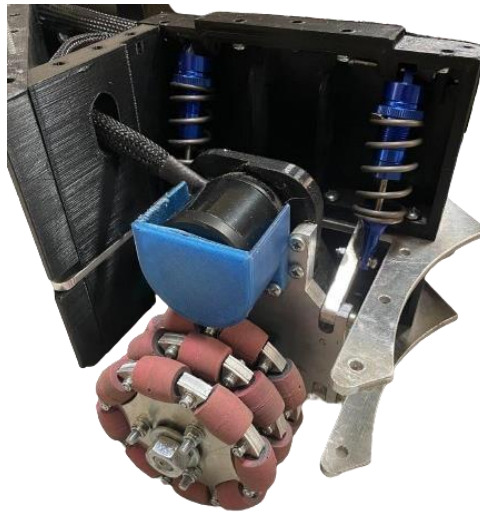
Fig. 3 . Suspended gearbox with omni-wheel
