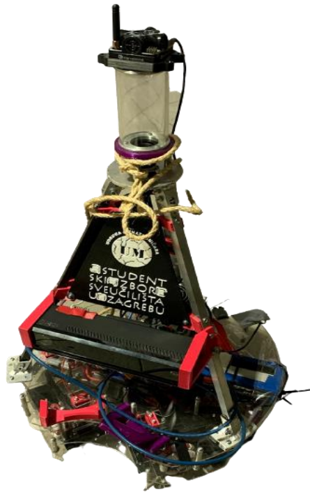
Fig. 1. Robot with active beacon on top
