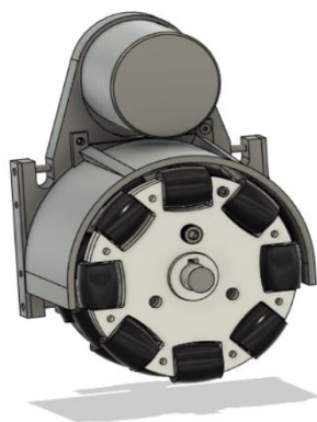
Fig. 2. Robot wheel with motor and dust cover
